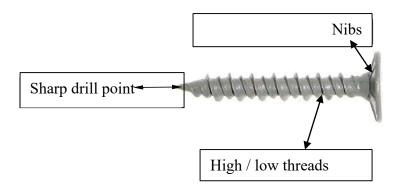
7.2.2 Fastening to metal, 18 gauge or heavier, with screws: Utilize a #8 or thinner shank flat head screw with nibs under the head for countersinking into the Magnum Board®, and a self-drilling point for penetrating the light gauge metal.
