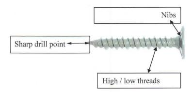
7.1.2 Fastening to metal, 18 gauge or heavier, with screw: Utilize a #8 flat head screw with nibs under the head for countersinking into the Framing, and a self-drilling point for penetrating the light gauge metal.
