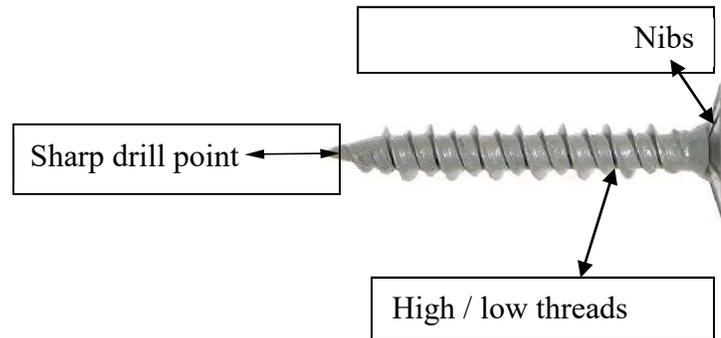
7.2.2 Fastening to metal, 18 gauge or heavier, with screw: Utilize a #10 flat head screw with nibs under the head for countersinking into the Magnum Board®, and a self-drilling point for penetrating the light gauge metal.
