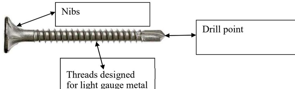
7.2.3 When fastening to light gauge materials lighter than 18 gauge, it may be necessary to utilize pneumatic fastening. Fasteners shown in 6.2.2 above may strip out lighter gauge studding prior to countersinking the head of the fastener into the Magnum Board® sheathing.
