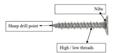
7.2.2 Fastening to metal, 18 gauge or heavier, with screw: Utilize a #8 flat head screw with nibs under the head for countersinking into the Magnum Board®, and a self-drilling point for penetrating the light gauge metal.
